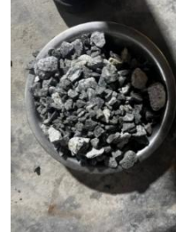
1b: Coarse Aggregate (crushed stone)
